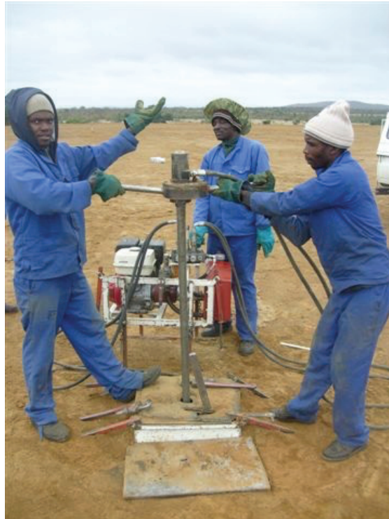
Figure 3. Auger drilling of a gold tailings dump.
